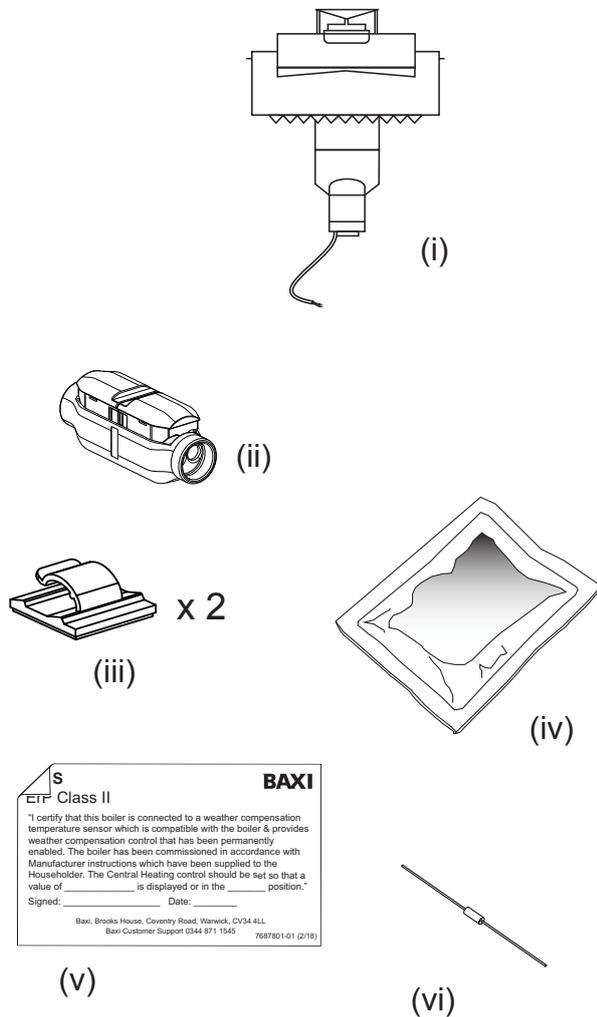
**IMPORTANT:** This kit is for use with vertical flue ridge terminals in a flue system of up to 4 metres actual length. A 5 metre sensor cable extension is available as an optional extra. The kit cannot be fitted where other devices such as the MULTIFIT GasSaver are incorporated into the flue system. It is permissible to shorten the cable. If shortening the cable DO NOT cut the sensor end !
